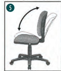
5 Tilt Pivot point located directly above center of chair base (white dot indicates pivot point).
