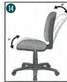
14 Auto Adjusting Synchro Tilt This self-adjusting control uses your weight to balance the force needed to recline the back. Back tilt is controlled by a single lever which will lock in 5 positions. When tilting, the seat tilts at a 4-to-1 ratio to the back.
