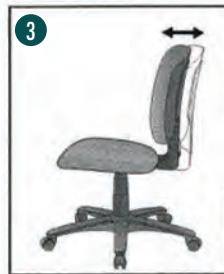
3 Seat Depth Adjustment Positions chair back relative to seat to reduce pressure on the buttocks and thighs for both taller and shorter users.
