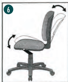
6 Mid-Pivot Knee Tilt Pivot point located slightly ahead of center of gravity (white dot indicates pivot point). Allows user to recline at a slightly more relaxed angle than conventional center tilt.
